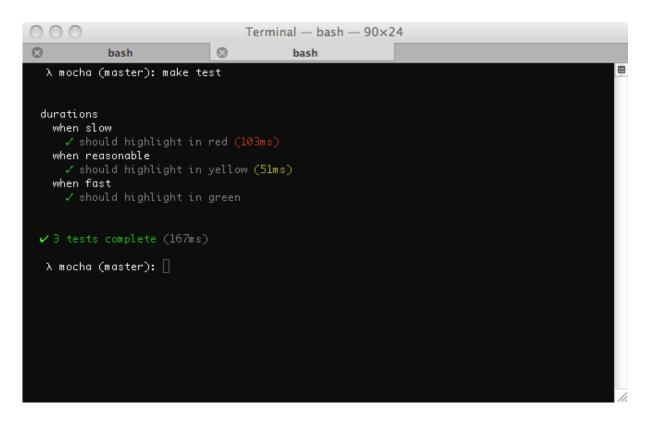
Figure 3.1: Mocha runner output in the command line
