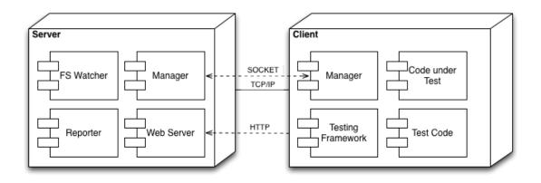
Figure 4.1: The high level architecture
